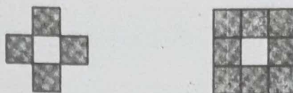
Fig. 11.10: Two definitions of a raster cell's neighbourhood. In the rooks case only the four cells that share an edge are neighbours, but in the queen's case the neighbourhood includes the four diagonal neighbours
